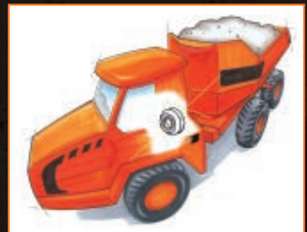
Turning ring placement in front of the articulation point provides equal weight distribution to the front wheels at all times.
